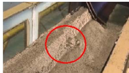
Figure 2.4 Bank erosion resulting from intermittent block failure
