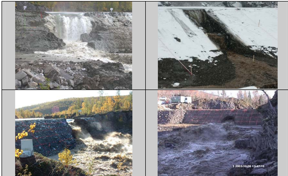
Figure 2.2: Breach development stages (4 different field tests)
