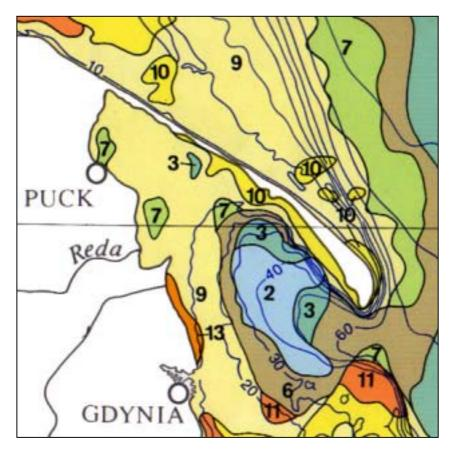
*Fig. 5: Surficial bottom sediments: (2) silty clay, (3) clayey silt,, (6) sand-silt-clay, (7) silty sand, (9) fine-grained sand, (10) medium-grained sand, (11) coarse-grained sand, (13) vain-grained sand. Source: Kramarska 1995.*
