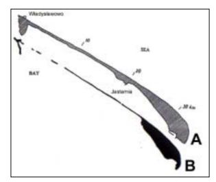
*Fig.9: Effect of expected sea level rise and storm surge on the shape of Hel Spit; A- mean sea level, B - +2.5 m. (Basinski 1995).*
