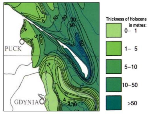
Fig.1: Thickness of Holocene deposits. Source: Geological Atlas of the Southern Baltic, 1995.
